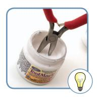
To protect the rings from any tool marks, use Tool Magic. This product provides a temporary rubber coating to your pliers. It is important to let it dry for at least 3 hours before using it. It is mostly recommended when working with aluminum rings.
